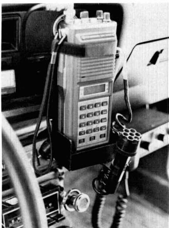
Handheld in ashtray mount makes a convenient mobile installation.
