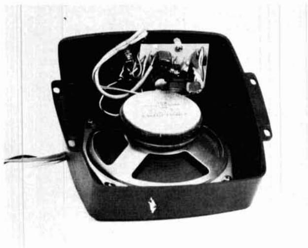
The audio amplifier is mounted inside the speaker enclosure using a metal stand-off post. The power and audio leads are secured with a plastic cable clamp.
