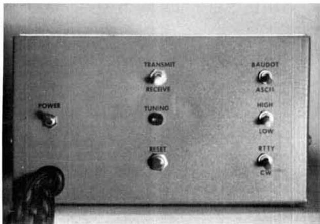
Front panel of the modem box. All switches are accessible. A tuning indicator is included, which is helpful when receiving narrowband signals on RTTY.
