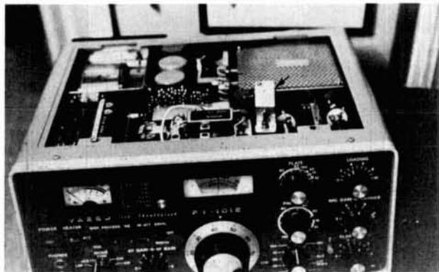
fig. 5. Photo of the preamp and switch assembled inside the FT-101 (arrows). Routing of the miniature coax cables is not critical and uses existing pass-through holes in the chassis.
